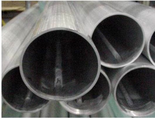
Fig. 4 Starting blank fabricated from a rolled and welded piece of sheet
