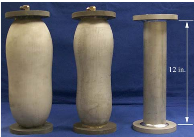
Fig. 9 Superplastically formed (SPF) free-expansion testing of AA5083 seamless tube samples
