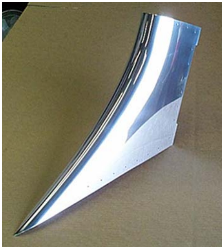
Fig. 11 Superplastically formed (SPF) 737 wing outboard leading edge strakelet
