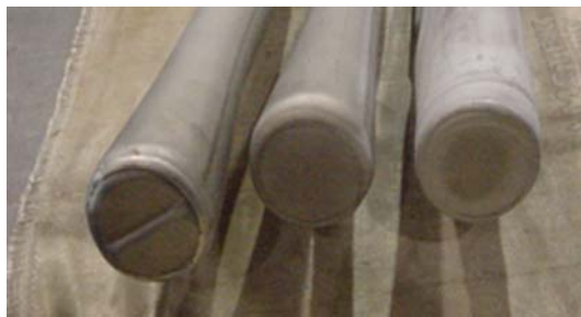
Fig. 5 End caps welded to part blanks
