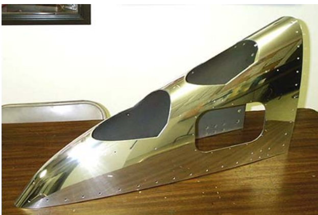
Fig. 13 Superplastically formed (SPF) AA5083 777 wing tip light housing
