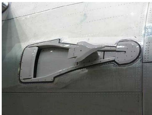
Fig. 2 2004 superplastically formed (SPF) 737 auxiliary power unit air inlet installed on the airplane
