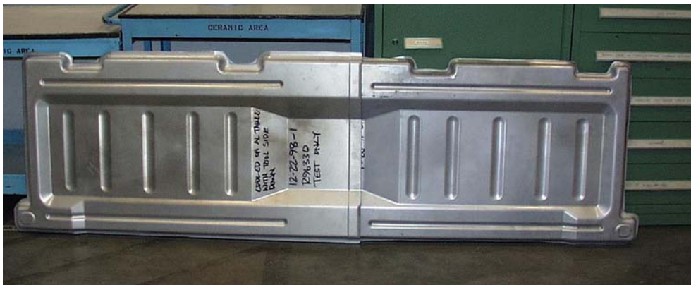
Fig. 10 767 superplastically formed (SPF) moisture shroud assembly comprised of two SPF AA5083 components
