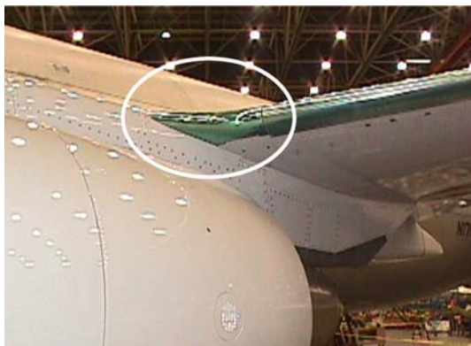
Fig. 12 Location of the superplastically formed (SPF) AA5083 strakelet on the 737 wing leading edge
